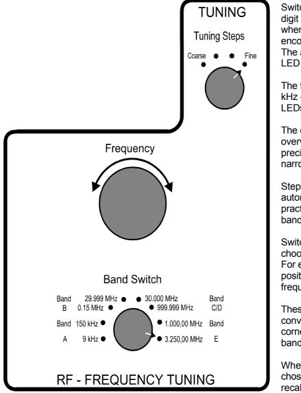
Switch TUNING selects the digit to tune the frequency when rotating the rotary encoder.
