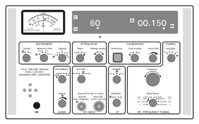
Step 2: Connect the r.f.- output of the l.i.s.n. to the receiver's left r.f. - input (bnc).
