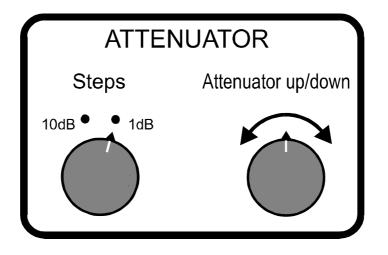
The field Attenuator serves for the control of the step attenuator. The step attenuator attenuates the input signal to a level which is appropriate for the receiver's front end.
