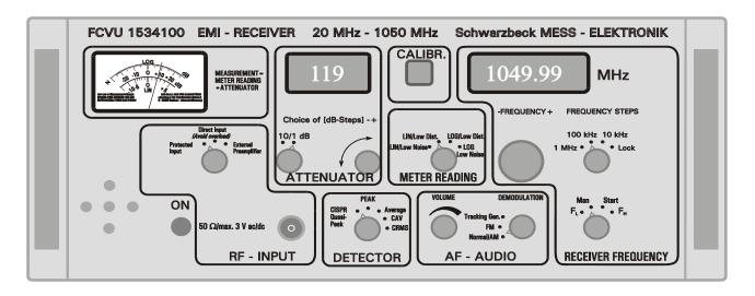
Interference measuring receiver for front panel operation with or without xy - recorder
