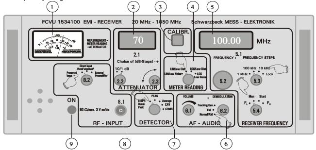
The receiver is now ready to use and frequency is tuned by rotating the encoder (5.2). The steps can be selected with (5.3).
