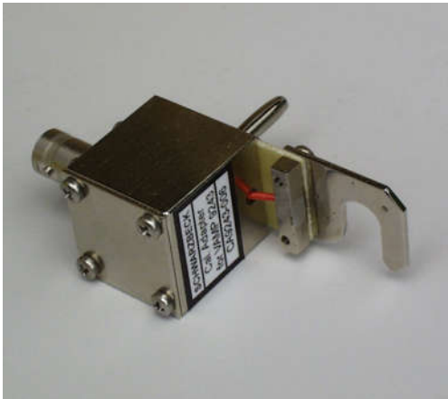
Fig. 9: Practical implementation of a source matched calibration adapter
